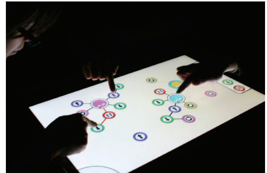
Fig. 1. RoboJockey interface; users coordinate robot performance by connecting action objects to robot objects.
