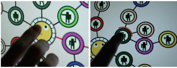
Fig. 10. Rotating a robot object with two fingers (left), Deleting child objects by holding down an object (right).
